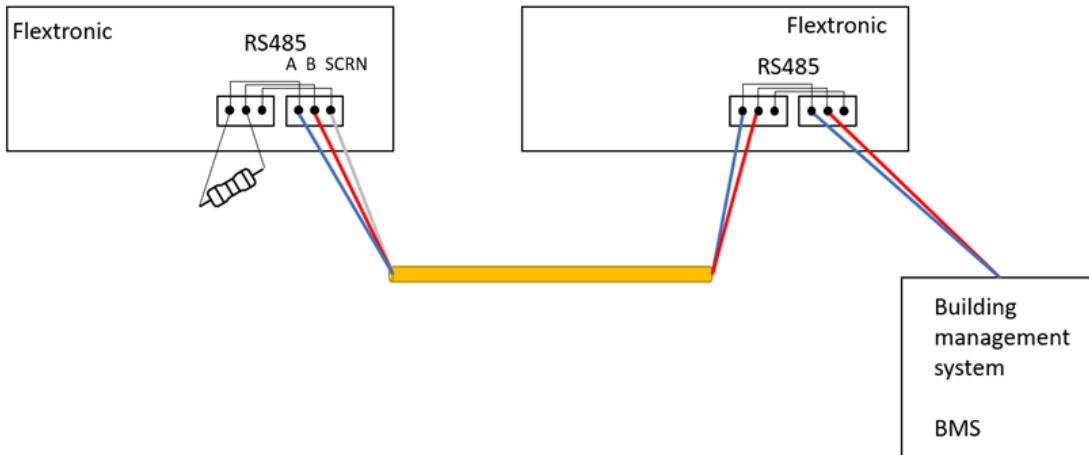
Communication as both Modbus and Bacnet is not possible on the RS-485 BUS at the same time. If both protocols are required, one of the protocols must run over the Ethernet connection (IP).
