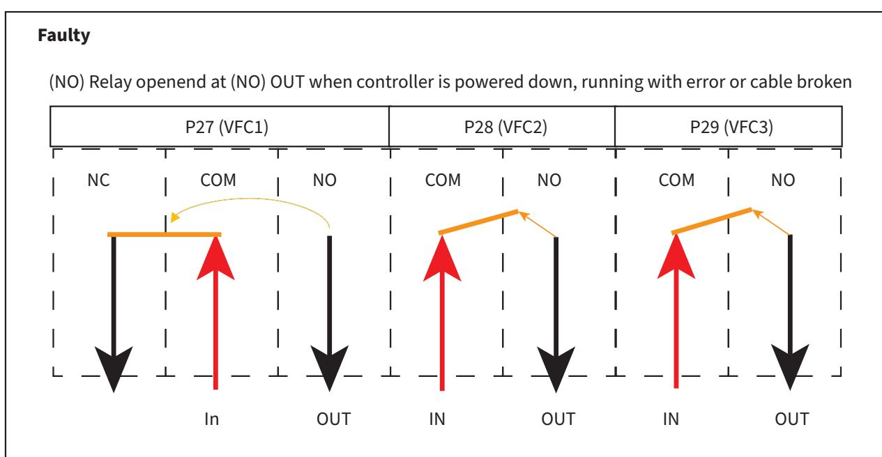
To acquire the status of the automat. The custom fault can be assigned to every output. Output P29 is a boiler interlock signal of the >110 °C mode, it is not available for alarming in this mode.
